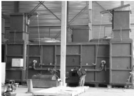
Figure 2 Front view of a Twin-retort carbonisation unit. Two carbonisation vessels are placed in the unit to function in tandem.
