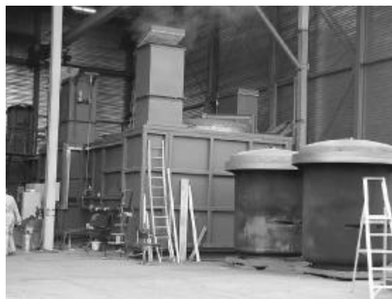
Figure 1 Side view of a Twin-retort carbonisation unit. To the right two carbonisation vessels are shown
